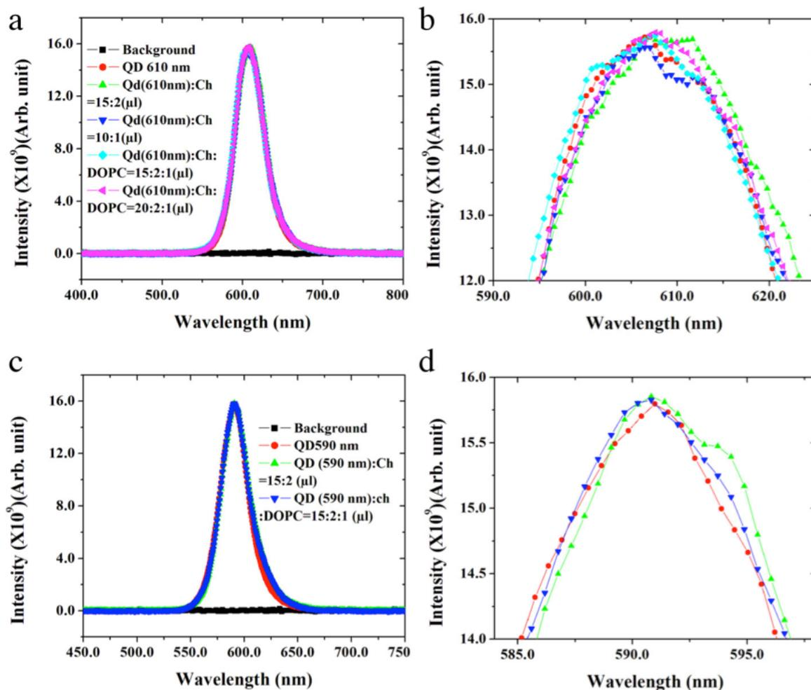
**Figure 3:** Photoemission spectra of CdSe/ZnS features. (a) Spectra of CdSe/ZnS (4.0 nm) features emitting at 610 nm. Different colours indicate the different ink compositions used. (b) Zoom-in of the data shown in (a). (c) Spectra of CdSe/ZnS (5.2 nm) patterns mixed with carrier inks emitting at 590 nm and (d) close-up of the peak area.
