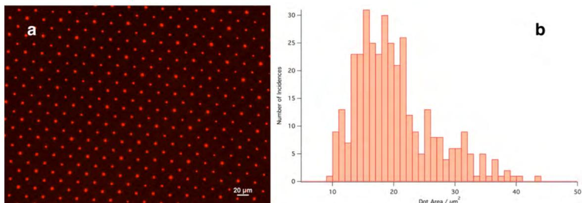
**Figure 4:** QD array by PPL. An ink composition of QD (4 nm): cholesterol 10:1 was used. **(a)** The fluorescence micrograph shows a part of a  $1 \times 1 \text{ cm}^2$  QD pattern. The spacing between the pens is 40  $\mu\text{m}$ . Each pen generated four spots. The stamp was automatically re-inked with a stamp pad after each approach. **(b)** shows the histogram of the dot area distribution of the dot pattern in (a). The average dot area was found to be  $(20.1 \pm 6.5) \mu\text{m}^2$ .
