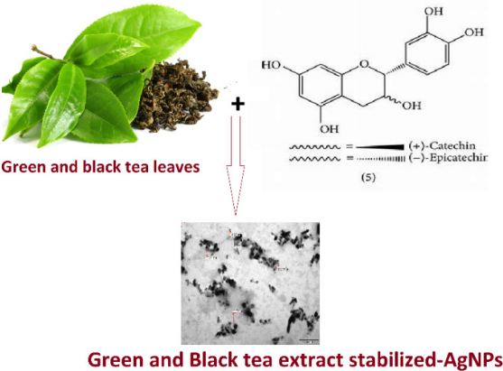
Figure 10. Tea stabilized green synthesis of AgNPs mechanism.
