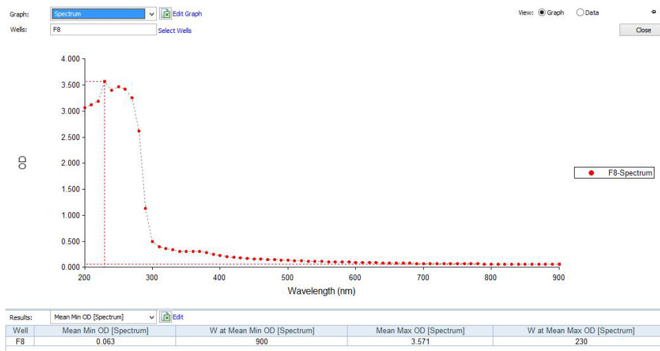
Figure 1. UV-Vis absorption spectra of commercially purchased CuO-NPs revealing \lambda_{\text{max}} at 230nm.
