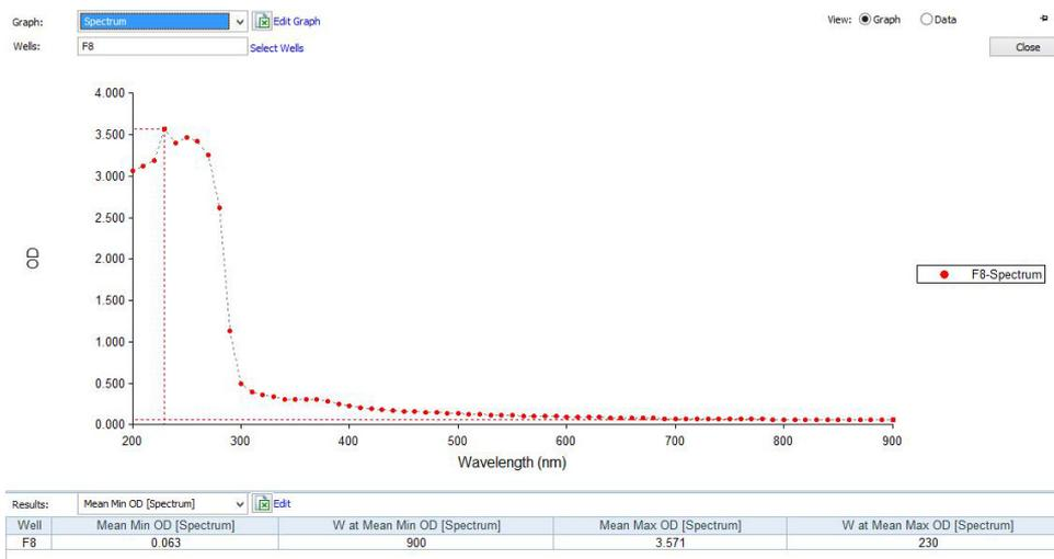
**Figure 1.** UV-Vis absorption spectra of commercially purchased CuO-NPs revealing  $\lambda_{max}$  at 230nm.
