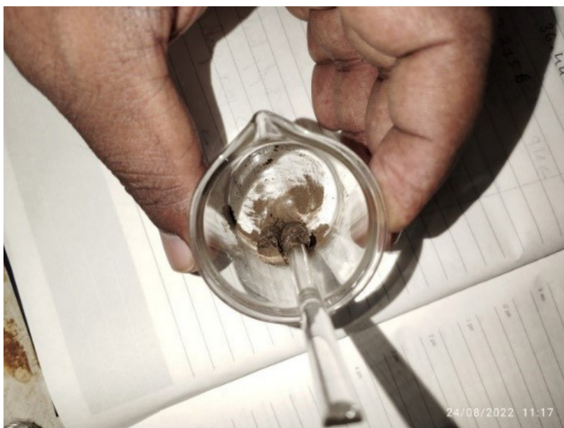
Figure. 1. Manual incorporation of Titanium oxide nanoparticles into Transbond XT composite.
